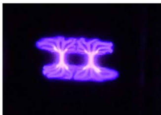
Fig. 1. The photo of two filaments on CDBD electrode in Ar/N 2 mixture at flow Ar: 0,31 l/min and N 2 : 0,1 l/min at frequency 3.36 MHz.
