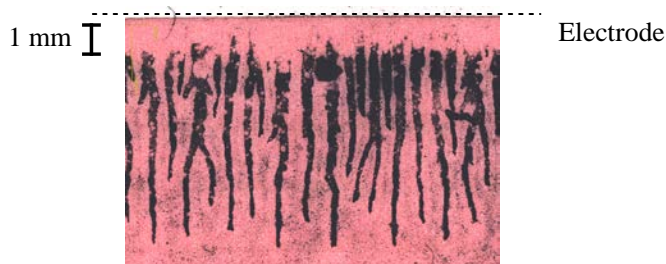
Fig. 2: Dust figure of the positive charge left on the ceramic barrier after impulse discharge
