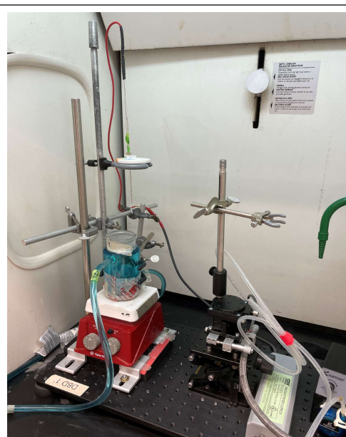
Figure 1—System for the degradation of methylene blue using CAPP.
